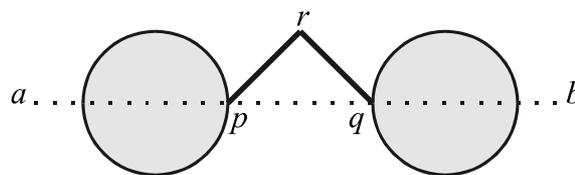
The sign consists of the two rods,  $[rp]$  and  $[rq]$ , described above, now rigidly jointed at  $p$  and  $q$  to two uniform discs, each of radius 0.2 m and mass  $M$  kg.
